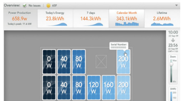
Screenshot of Enphase's data monitoring app, which reports the wattage produced by each module.
